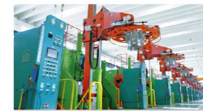
液压系统热板式双模硫化机 Hydraulic system hot plate dual-mode vulcanizing machine
